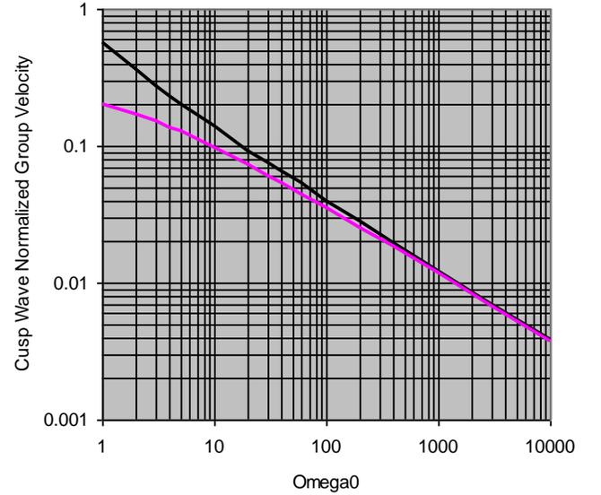
Fig. 4. The normalized group velocity of cusp waves as a function of  $\Omega_0$  for positive frequencies (—) and negative frequencies (—).
