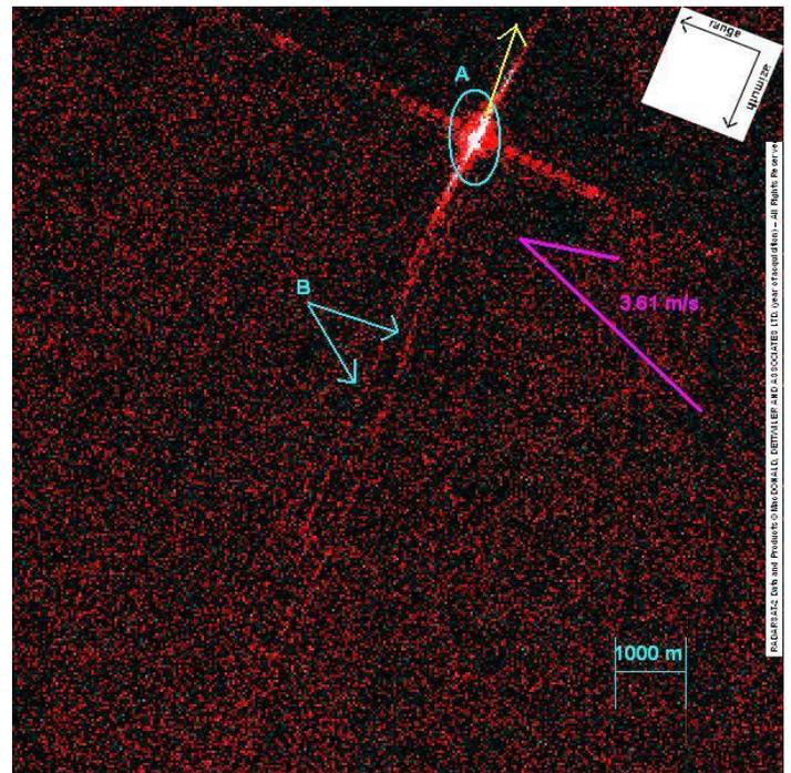
Fig. 1. Image of the Westwood Rainier and its narrow-V wake. A: ship return. B: narrow-V wake arms. (From Roy [1].)
