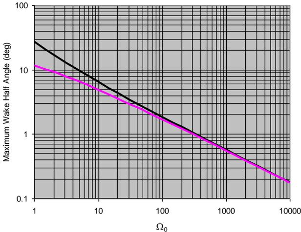
Fig. 3. The wake half angle as a function of  $\Omega_0$  for positive frequencies (—) and negative frequencies (—).
