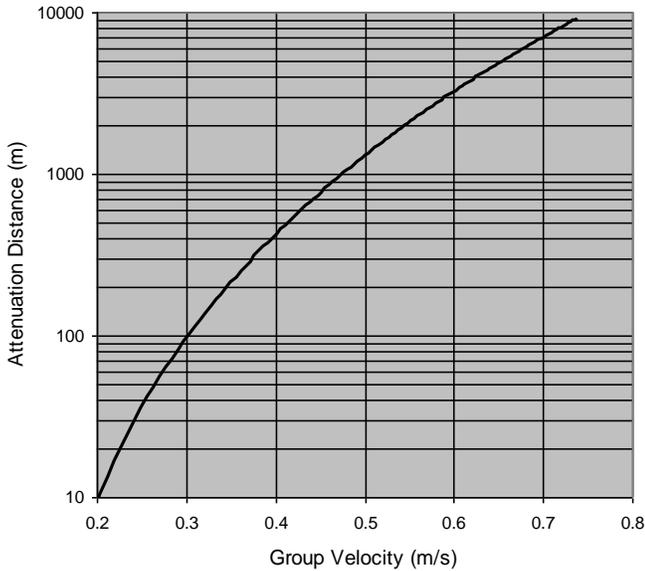
Fig. 5. The attenuation distance as a function of group velocity.
