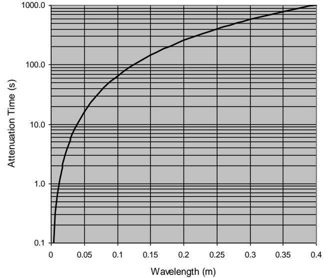
Fig. 2. The attenuation time due to viscous damping as a function of wavelength.
